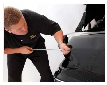
Working on a rear fender dent through the taillight opening. (Image: Dent Wizard)
