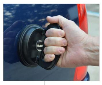
A suction cup puller being used for dent removal. (Image: AAA)
