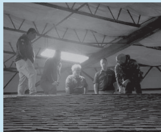
COLLAGE OF ADVANCED ROOFING CERTIFICATION STUDENTS USING HAIL CANNON AND EVALUATING THE RESULTING DAMAGE TO ROOF SHINGLES
