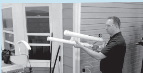
COLLAGE OF ADVANCED ROOFING CERTIFICATION STUDENTS USING HAIL CANNON AND EVALUATING THE RESULTING DAMAGE TO ROOF SHINGLES
